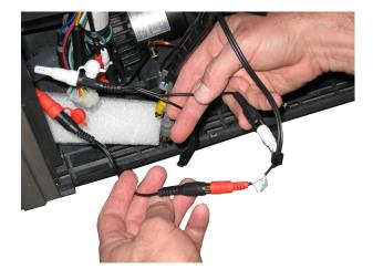
Attach the Red and White Audio cables from the TV to the corresponding Audio Y cables.
