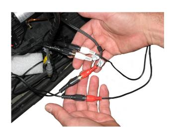
Attach TV Power cable to the APM Module Using one black, white and green connector.
