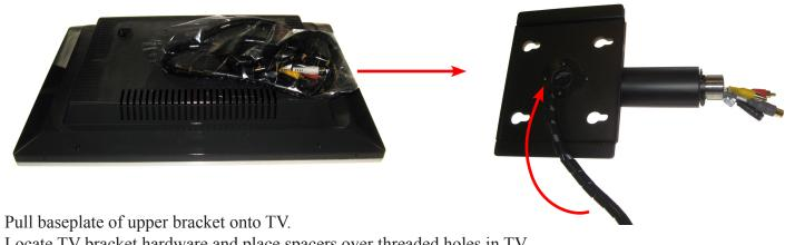
Locate TV bracket hardware and place spacers over threaded holes in TV.
