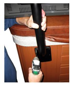
Attach the lower bracket with TV back onto the spa making sure the wires have been pulled completely through the 1" hole.
