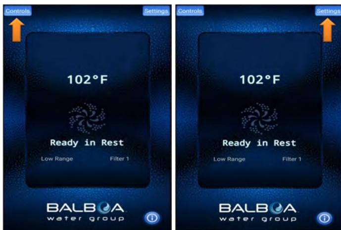
Selecting "Controls" will open a list of installed components like pump(s), blower, lights, etc.
