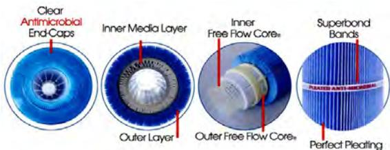
The outer core is similar to a traditional filter which traps larger debris, while the inner core filters the water for particles down to 3 microns in size. The inner core is easily removed and both filter media can be cleaned.
