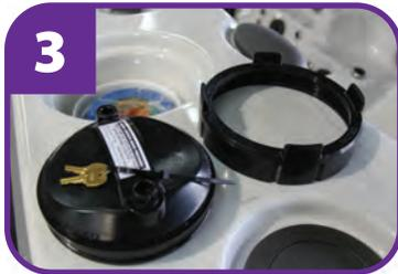
Remove the filter lock ring and lid. Remove filter and take it out of the plastic transport bag.
