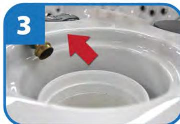
Remove fill hose from filter canister.
