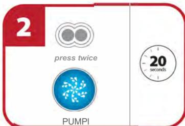
Turn pump 1 on high speed for 20 seconds by pressing the pump icon twice.
