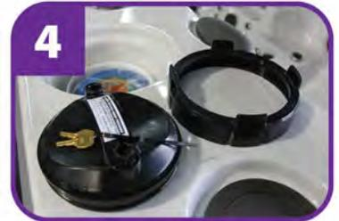
Remove the filter lock ring and lid.
