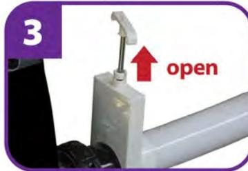
Ensure that any gate/knife valves are fully open.
