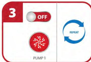
Turn pump 1 off by pressing the pump one icon once. Repeat steps 2 and 3 until air is removed from pump 1 and water is coming from jets.
