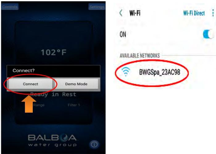
**Step 4:** Once connected to the Wi-Fi Module directly open the Coast Spas app. The Coast Spas app will allow you to control and interact with the spa while you are still with in range.
