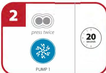
Turn pump 1 on high speed for 20 seconds by pressing the pump icon twice.
