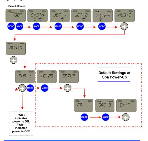
\*IMPORTANT: Ten seconds is required during power activation to allow the system to preset the default settings for Volume, EQ, and SRC.
